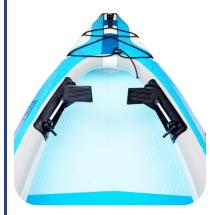
Repeat pedal installation on the other side. Pedal positions are numbered for easy alignment. Adjust pedal while on the water by lifting pedal with a foot and slide pedal fore or aft.
