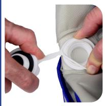
Stretch retainer ring over the valve base. Retainer ring fits in a groove in the valve base. Screw valves into bases. Tighten valves firmly so air does not escape while sitting on seat. Unscrew cap for inflation.
