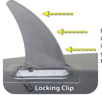
Flip boat over and slide skeg into skeg base. Skeg must go in far enough for locking clip groove to line up with slot in the skeg.
