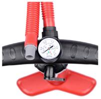
To inflate the seat screw the hose with wide-mouthed cone-shaped adapter into the pump handle by twisting the collar onto the threaded opening in the pump handle until hose is tight (about 1/8 turn).
