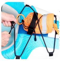
The cargo hold-down elastic straps at the front and back of the kayak are adjustable. To adjust, pull on the free end until cord comes out of jamb clip. Adjust length and pull the cord down into the locked position
